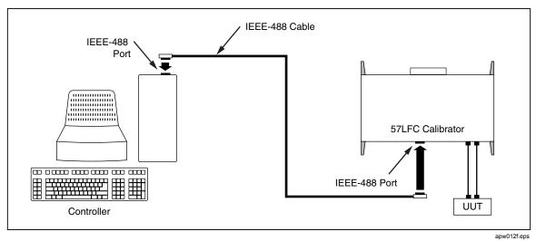
Figure 3-3. Testing the IEEE-488 Port
