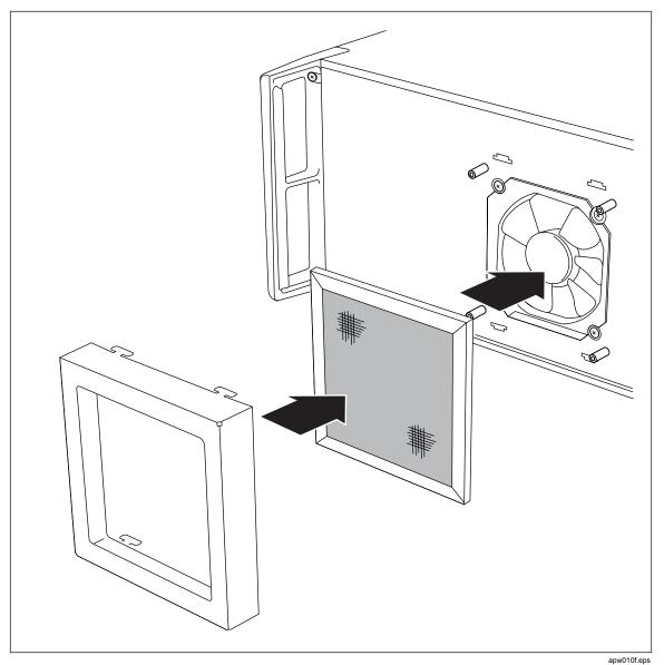
Figure 4-2. Accessing the Air Filter
