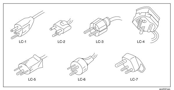
Figure 2-4. Line Power Cord Types Available from Fluke
