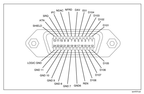
Figure 3-2. Typical IEEE-488 Remote Control Connections
