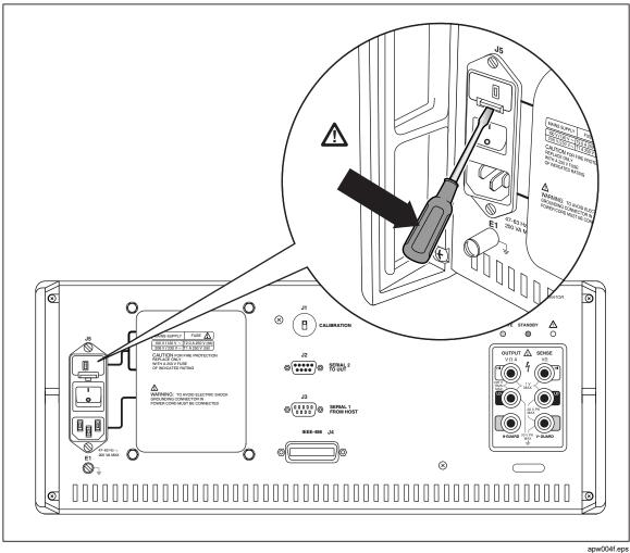
Figure 4-1. Replacing the Fuse
