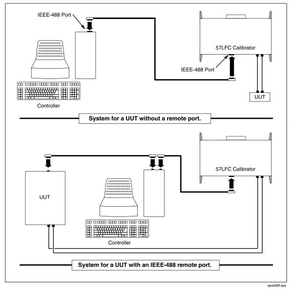
Figure 3-1. Typical IEEE-488 Remote Control Configuration
