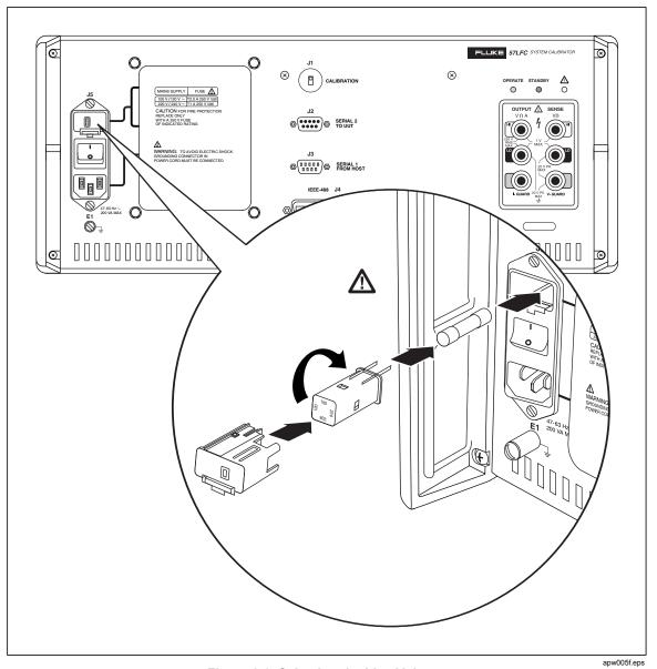
6. Install the fuse holder in the calibrator.
